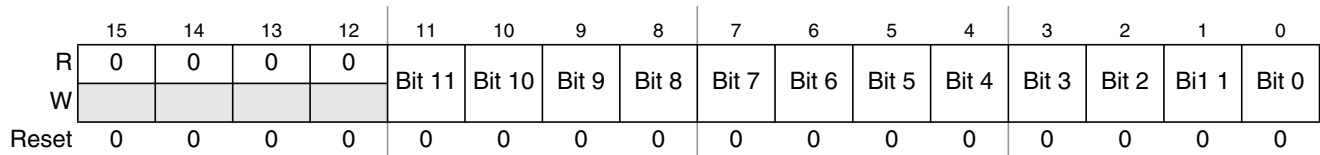
Figure 13-15. Right justified ATD conversion result register (ATDDR n )
