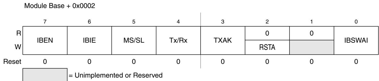
Figure 15-6. IIC Bus Control Register (IBCR)
