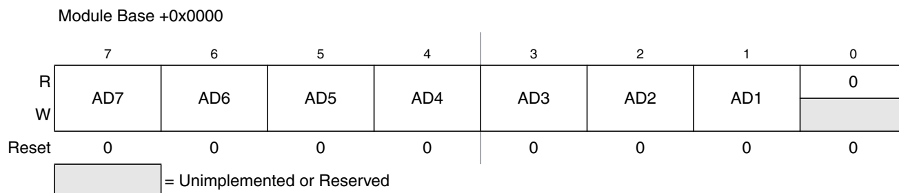
Figure 15-3. IIC Bus Address Register (IBAD)
