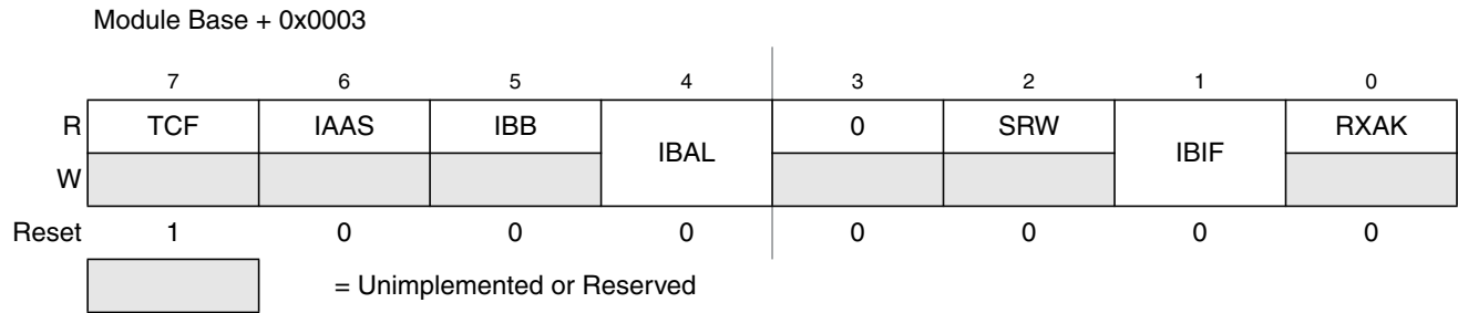
Figure 15-7. IIC Bus Status Register (IBSR)
